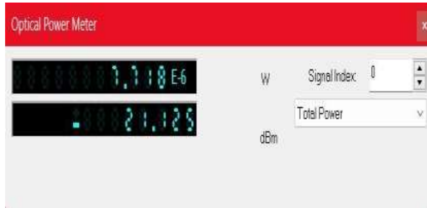
Figure 8. The result of the Link Power Budget (LPB) testing for the Fiber To The Area network
