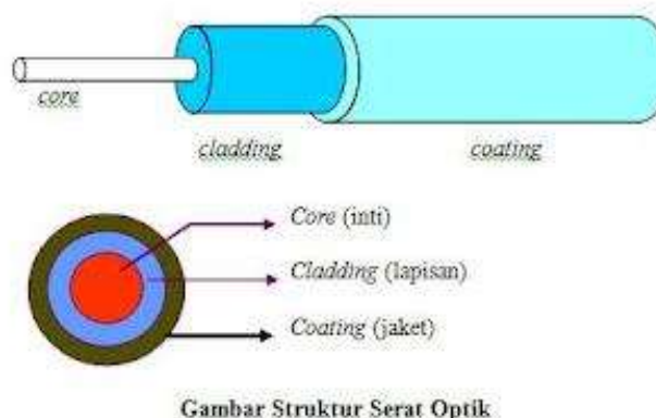
Figure1. The Structure of Optical Fiber
